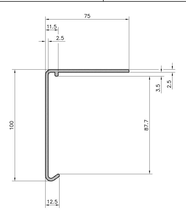
SUPPLIED IN 2.5 METRE LENGTHS WITH LOOSE JOINTING SLEEVE 90° INTERNAL AND EXTERNAL CORNER PIECES AVAILABLE STANDARD COLOURS BLACK, WHITE AND GREY OTHER COLOURS CAN BE SUPPLIED, PRICES & LEAD TIMES ON APPLICATION
