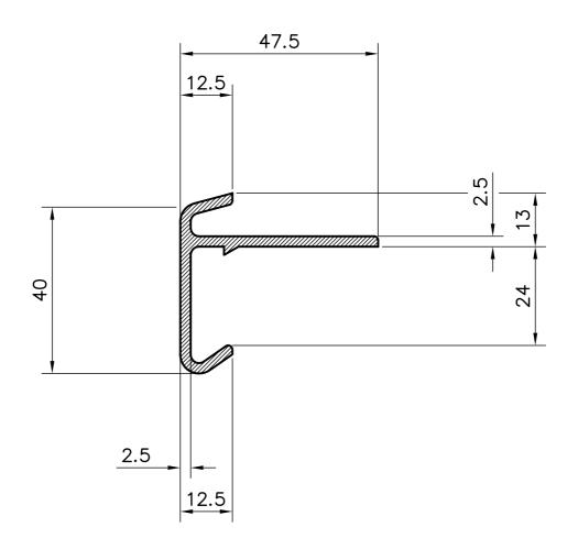
SUPPLIED IN 2.5 METRE LENGTHS WITH LOOSE JOINTING SLEEVE 90° INTERNAL AND EXTERNAL CORNER PIECES AVAILABLE STANDARD COLOURS BLACK, WHITE AND GREY OTHER COLOURS CAN BE SUPPLIED, PRICES & LEAD TIMES ON APPLICATION
