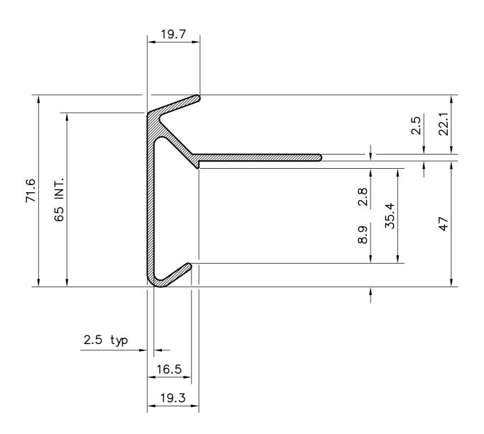
SUPPLIED IN 2.5 METRE LENGTHS WITH LOOSE JOINTING SLEEVE 90° INTERNAL AND EXTERNAL CORNER PIECES AVAILABLE STANDARD COLOURS BLACK, WHITE AND GREY OTHER COLOURS CAN BE SUPPLIED, PRICES & LEAD TIMES ON APPLICATION
