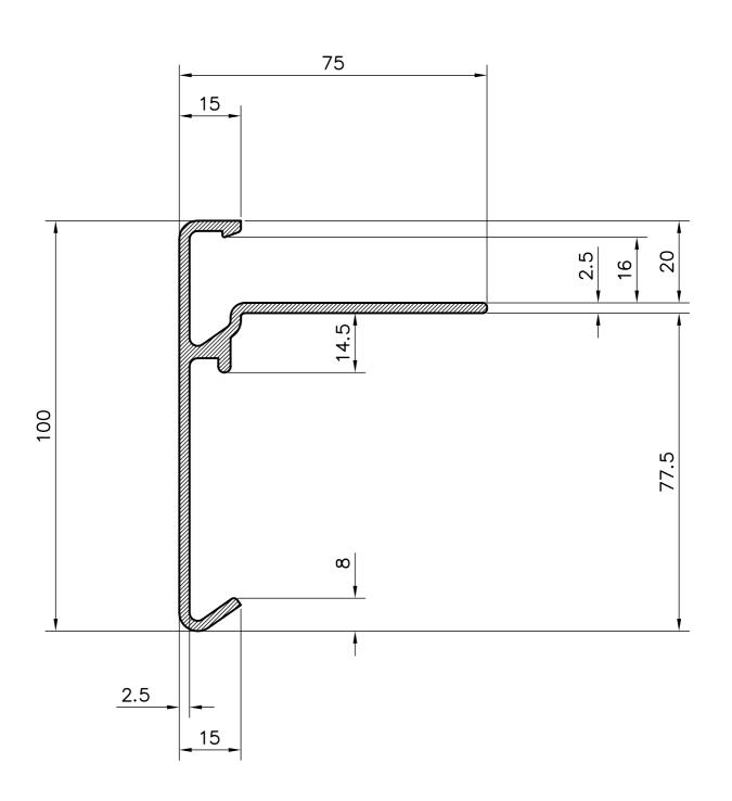
SUPPLIED IN 2.5 METRE LENGTHS WITH LOOSE JOINTING SLEEVE 90° INTERNAL AND EXTERNAL CORNER PIECES AVAILABLE STANDARD COLOURS BLACK, WHITE AND GREY OTHER COLOURS CAN BE SUPPLIED, PRICES & LEAD TIMES ON APPLICATION
