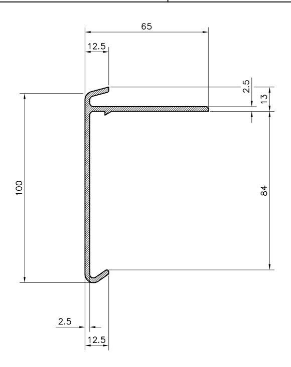
SUPPLIED IN 2.5 METRE LENGTHS WITH LOOSE JOINTING SLEEVE 90° INTERNAL AND EXTERNAL CORNER PIECES AVAILABLE STANDARD COLOURS BLACK, WHITE AND GREY OTHER COLOURS CAN BE SUPPLIED, PRICES & LEAD TIMES ON APPLICATION
