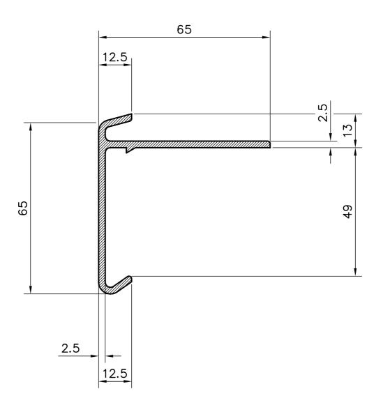
SUPPLIED IN 2.5 METRE LENGTHS WITH LOOSE JOINTING SLEEVE 90° INTERNAL AND EXTERNAL CORNER PIECES AVAILABLE STANDARD COLOURS BLACK, WHITE AND GREY OTHER COLOURS CAN BE SUPPLIED, PRICES & LEAD TIMES ON APPLICATION
