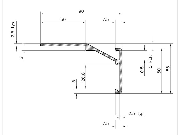
SUPPLIED IN 2.5 METRE LENGTHS WITH LOOSE JOINTING SLEEVE 90° INTERNAL AND EXTERNAL CORNER PIECES AVAILABLE STANDARD COLOURS BLACK, WHITE AND GREY OTHER COLOURS CAN BE SUPPLIED, PRICES & LEAD TIMES ON APPLICATION
